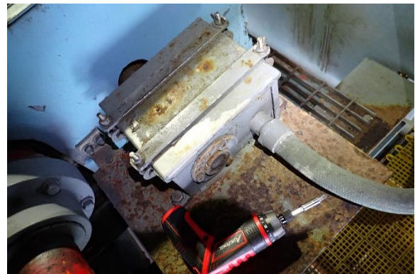
Photo 03: Corrosion on Rotary Cam Housing (Personal Photo)
